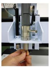
With small brush, clean the chips and particles from the inner surface of the collet chuck.
