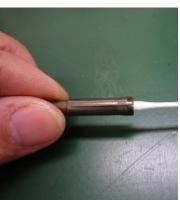
Make sure that no chips and particles are left behind in the slit of the collet chuck.
