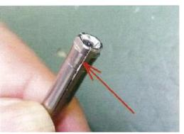
Also, you need to clean the inner side of the spindle motor housing using brush and cotton swab with small amount of alcohol.
