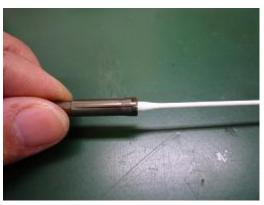
Make sure that no chips and particles are left behind in the slit of the collet chuck.
