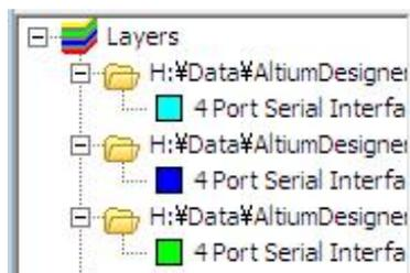
All of the Gerber files should appear on the workspace and the layer name added to the layer tree on the left side.
