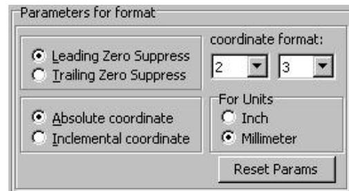
Instead of entering the settings by yourself, click **Autodetecting** to detect the most suitable parameters of drill format according to the Gerber pattern which is imported previously.
