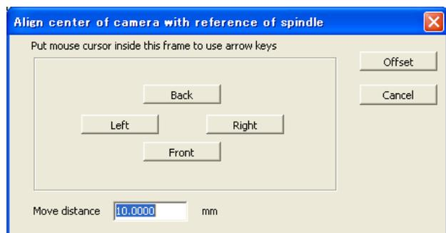
Move the camera to the location where the marker display matches the milling mark at P1.
