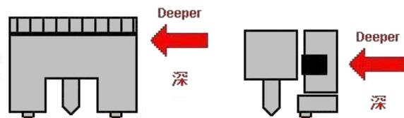
Confirm the tip of tool touch the board surface.
