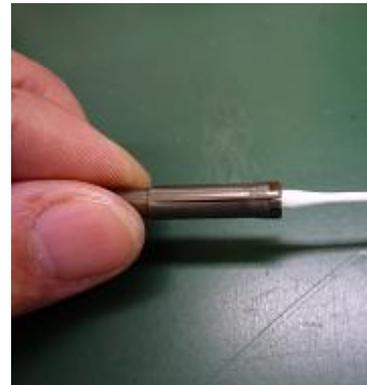
Make sure that no chips and particles are left behind in the slit of the collet chuck.
