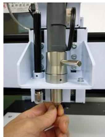
With small brush, clean the chips and particles from the inner surface of the collet chuck.
