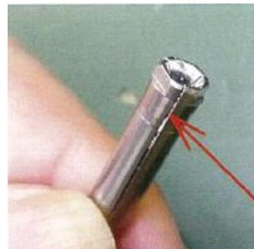
Also, you need to clean the inner side of the spindle motor housing using brush and cotton swab with small amount of alcohol.
