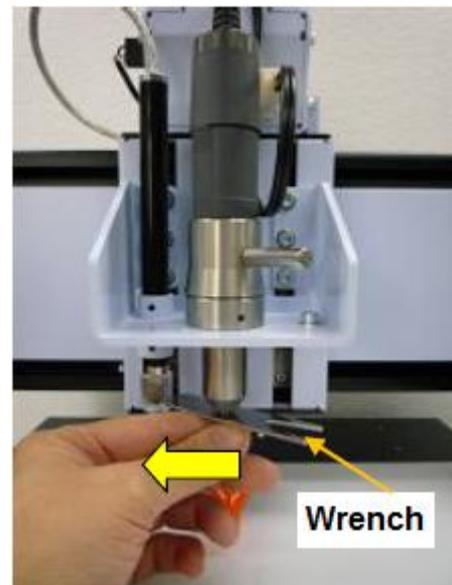
Once it is loosened, the collet chuck can be easily rotated with your fingers.
