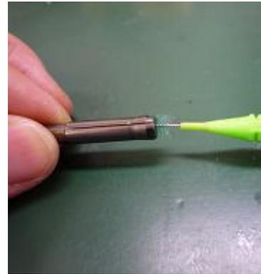
Apply small amount of alcohol on the cotton swab. Wipe with it and remove the oil and grease from the inner and outer surface of the collet chuck.
