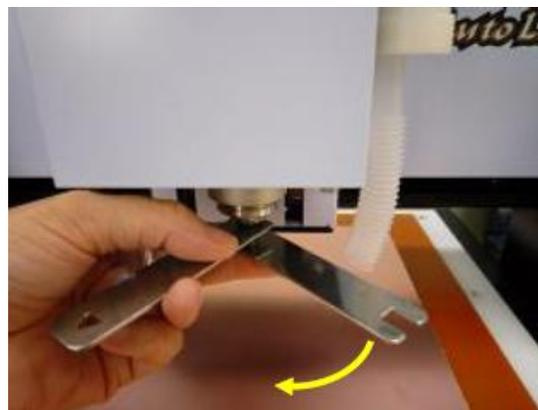
Once it is loosened, the collet chuck can be easily rotated with your fingers.
