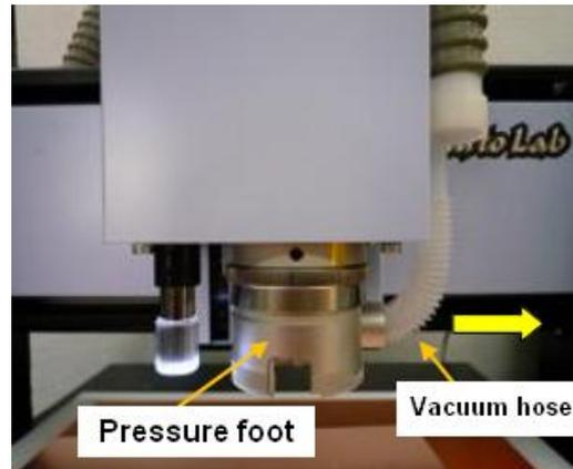
The pressure foot is fixed on the head assembly with 2 screws.:
