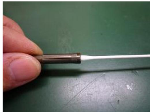
Make sure that no chips and particles are left behind in the slit of the collet chuck.
