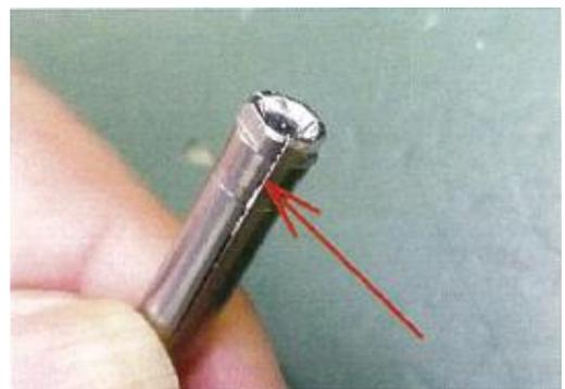
Also, you need to clean the inner side of the spindle motor housing using brush and cotton swab with small amount of alcohol.
