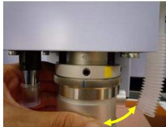
Finally when it reaches the top, make sure the yellow label of the pressure foot as shown in the right picture meets another label on the head assembly.
