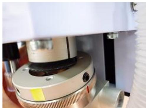
Push up the pressure foot shaking it left and right.
