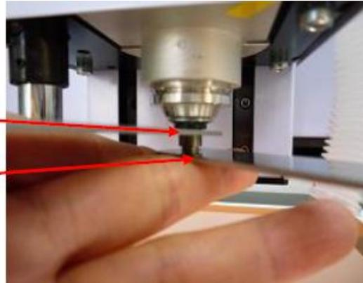
Holding the upper wrench, turn another wrench clockwise in a way of arrow as shown in the right picture. The collet chuck is going to be loosen.
