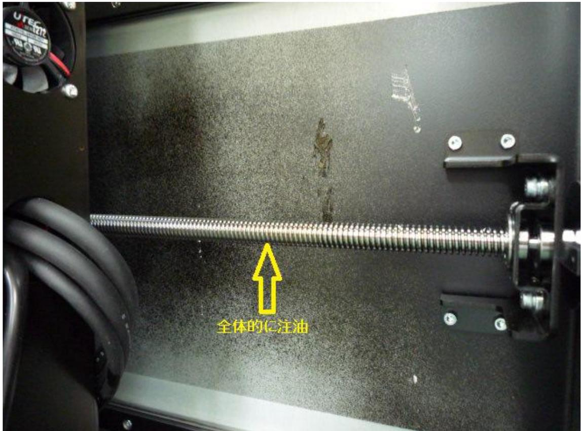
Another way is that you will put the oil from the slit of the left side or right side of the machine. Long stick is necessary to reach Y axis lead screw.
