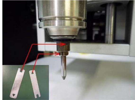
Using the special wrenches, apply rectangular jaw to the upper notch and the triangular hole to the bottom of the collet chuck as shown in the picture below.
