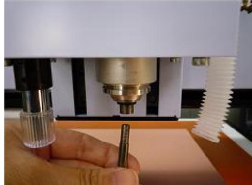
With small brush, clean the chips and particles from the inner surface of the collet chuck.
