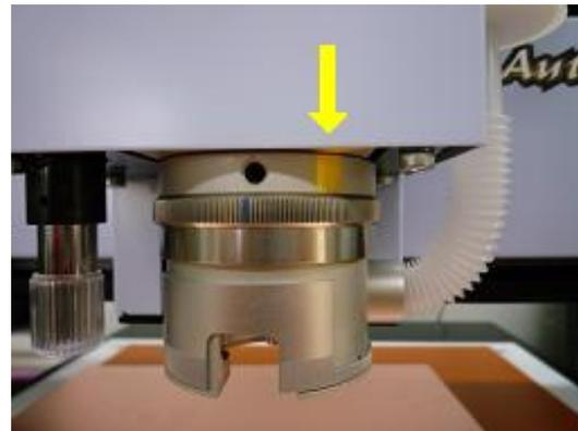
Then secure the set screws of the foot and attach the vacuum hose to the foot.
