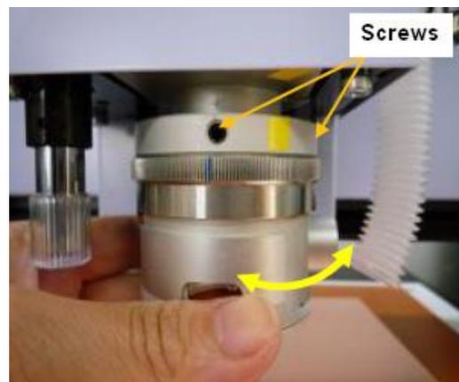
When the pressure foot is removed successfully, you will see the part of spindle motor, tool and collet.
