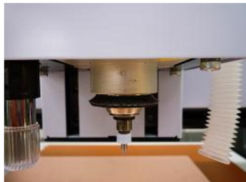
Make sure the set screws don't come out of the inner side of the pressure foot.
