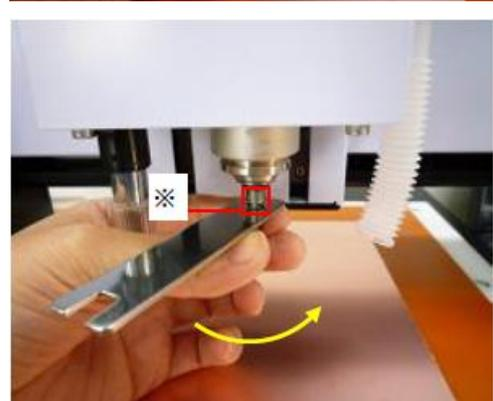
Insert dummy tool with ring instead of tool without ring.
